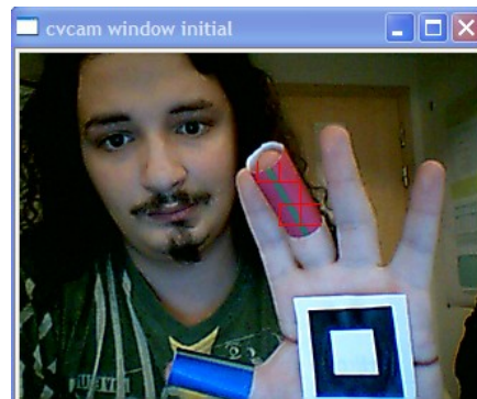
Figure 5: Grid-edge detection applied to webcam image. Edges complying with the threshold are colored in red (middle finger).
