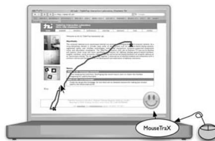
Figure 2. Schematized future eMotion system. The mouse tracking system records the mouse movements, enabling the application to react on user actions. Here, the system visualizes tracked data and user emotional state (smiley).
