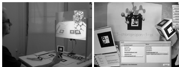
Figure 1. AC system with back-projection screen (left). TUI and GUI working at the same time: the rotation cube is operated with the right hand while the constructed molecule sits on the centre platform (right).
